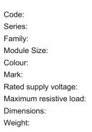
D5212.17 **CUBE** Series Integral Sockets Two Module **Charcoal Black** Norisys 240V 6A 60.0mm x 52.2mm x 35.5mm 89.10g
