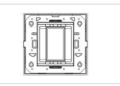
Code: Series: Family: Module Size: Colour: Mark: Rated supply voltage: Maximum resistive load: Dimensions: Weight: C5101 .16 CUBE Series Smart plates with frames One Module Matt Gold Norisys ----89.5mm x 92.4mm x 14.4mm
