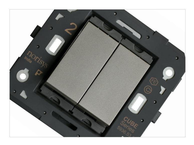
The bi-material support frames in CUBE Series is the result of several man-hours of research and development. The bi-material frames are made of a combination of steel and engineering grade plastic. In this design, a steel structure is embedded into plastic. The steel inside gives the bi-material frame a rigid structure while the plastic provides the antirust and insulation properties.
