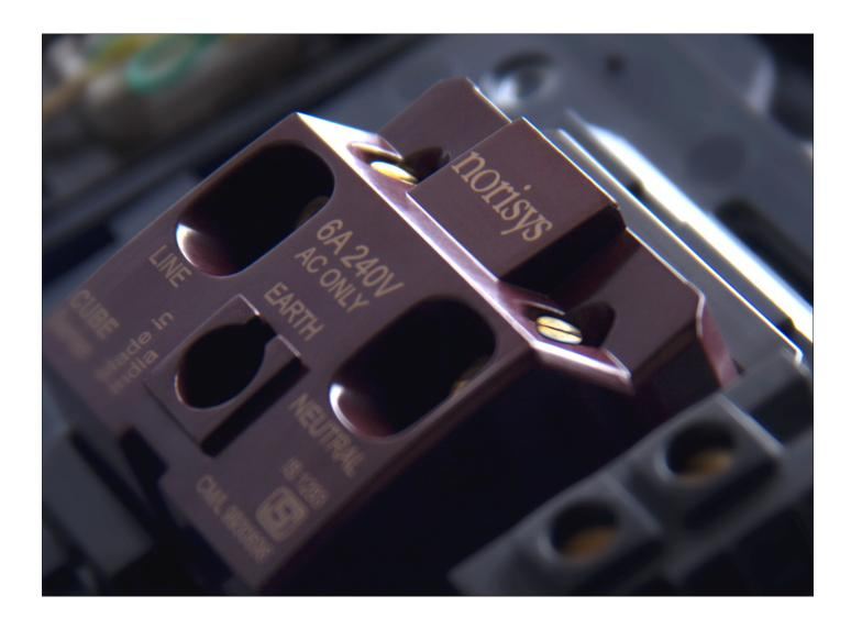
Modules such as switches, sockets etc. are made to a standard size (module) which are mounted on frames. Front plates are available in a variety of colours, materials and finish. The front plates can be changed at any time without disturbing the wiring to adapt to changes in building interiors.
